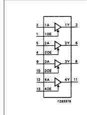
Fig.4 Functional diagram.
