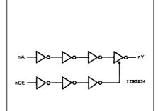
Fig.5 Logic diagram (one buffer).
